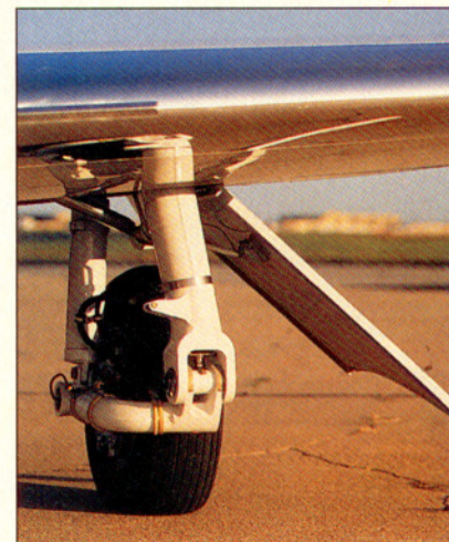
The CitationJet uses thrust attenuators instead of heavy, expensive reversers. Trailing-link gear aids in smooth landings.
